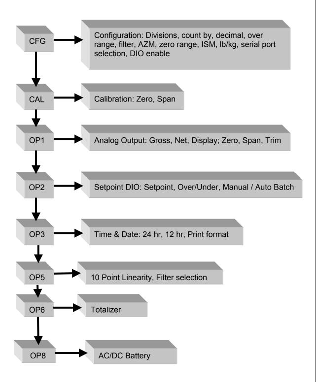
**CONFIGURATION: "SEL.CFG"** Use Zero to enter the menu and step to each category, Gross/Net to select parameters. Print to return to menu selection.
