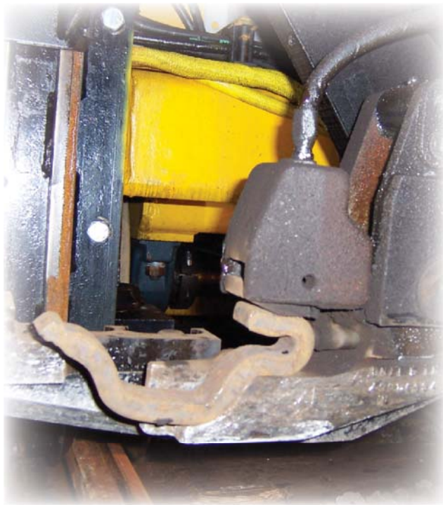
The anchor holders hold anchors firmly in place until the anchor application cycle is started.
