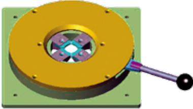
**Universal Bottle Holder (optional)** – The universal holder is designed to accommodate a range of finish sizes with the same fixture, eliminating the need to replace inserts for job changes. This option is ideal for applications with frequent job changes that involve bottles with varying neck and locking ring diameters.
