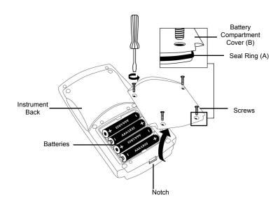
To ensure that the instrument is waterproof:
