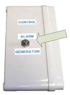
Use the toggle switch on the side of the R-20 Relay to select the operating mode desired.
