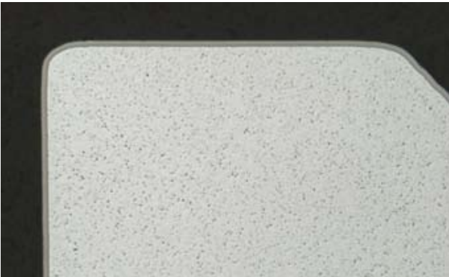
Uniform deposition of DNC-AL layer
