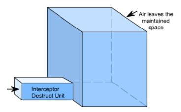
Method 2a; (Interceptor is placed directly inside of a small chamber or room)
