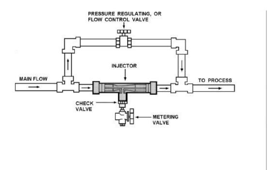
Bypass Assemblies should be installed so that the injector outlet is at, or above, the horizontal. "Full Flow" valves and pipe fittings should be used so that water flow through the injector is not restricted. Bypass Assemblies are available from Mazzei Injector Corporation in standard pipe sizes from ½ to 2". Custom manifolds are available in sizes to 8".
