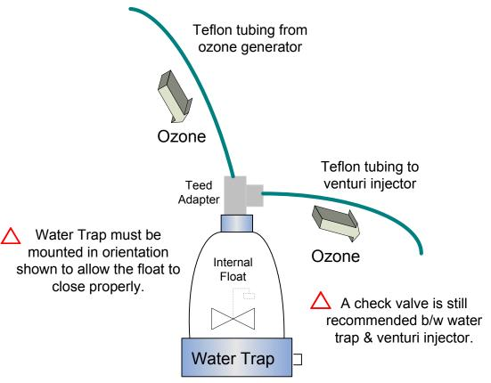
Ozone gas travels from the ozone generator through the teed adapter and into the horizontal Teflon tubing. The closed valve (not shown) on the water trap prevents ozone from escaping into the atmosphere.
