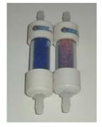
The MI-1moisture indicator (left) will alert you to when the AD-500 requires regeneration. The indicator on the left is blue which means that the air is very dry, and suitable for ozone generation. The MI-1on the right is purple/pink, which means that the AD-500 media must be regenerated. The MI-1 moisture indicator itself does not need to be regenerated, as it will revert to a blue color once the air having been dried by the AD-500 passes through it.
