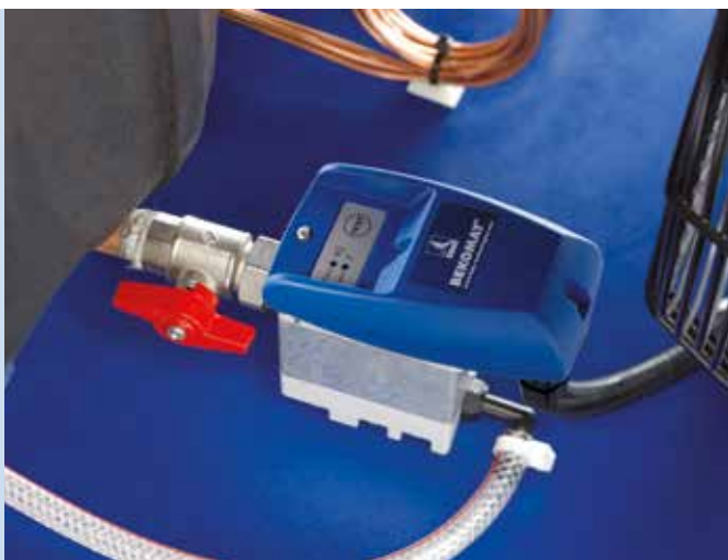
Condensate drainage without compressed air losses DRYPOINT® RA refrigeration dryers are equipped as standard with the electronically level controlled BEKOMAT® condensate drain.
