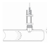
Insertion Depth = 1/8 of Pipe Inner Diameter
