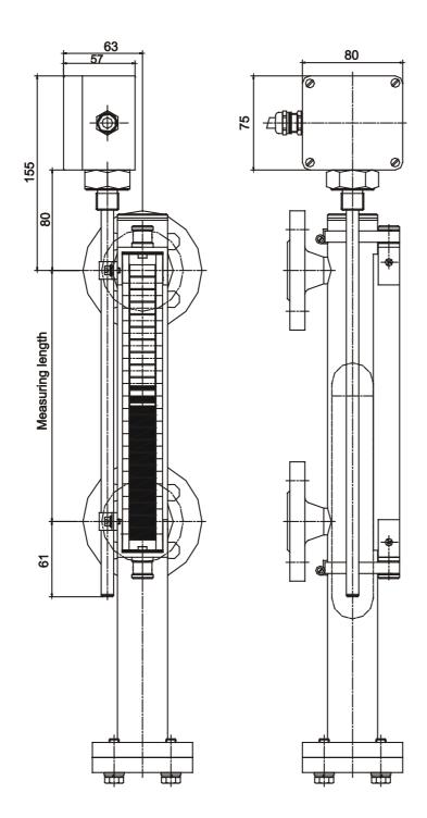
NBK-M with roller indicator and magnetostrictive transmitter
