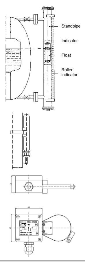
Remove bottom flange from bypass tube, and insert the cylindrical float in the NBK bypass tube with the designation "TOP" at the top. Re-position the gasket and close the bottom flange again; firmly tighten with screws. Mount and tighten the bypass tube to the vessel to be monitored with process connection and seal.
