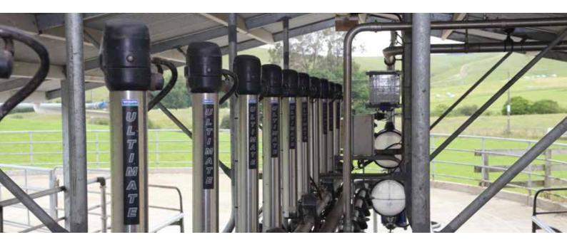
The Ultimate electronic cup remover is a reliable general purpose cup remover solution, designed to provide fast and efficient milking while reducing labour costs.
