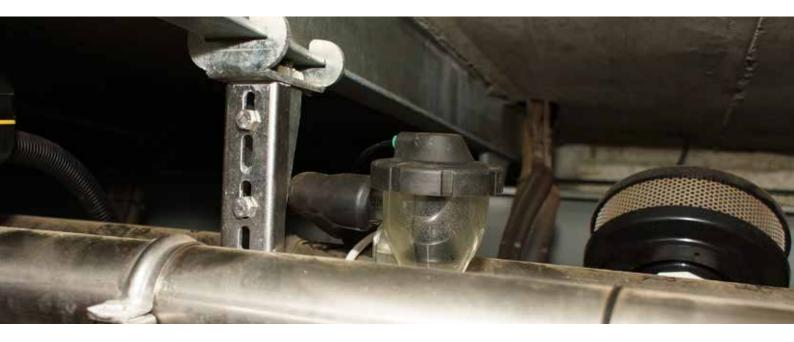
Vortex flow sensors work with Smart ECRs (cup remover technology) to accurately identify end of milking and maintain vacuum stability - even under the highest milk flow rates.
