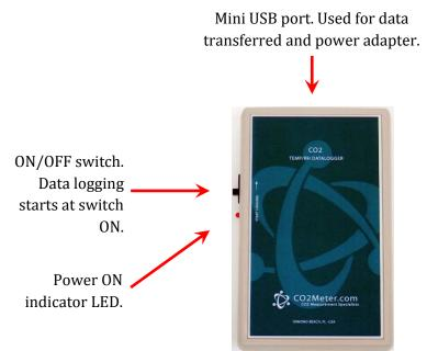
Figure 1: Data logger models without display
