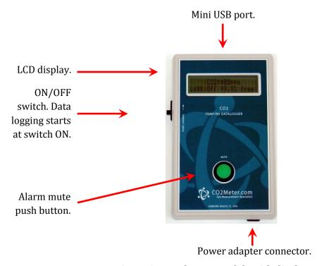
Figure 1: Data logger models with display
