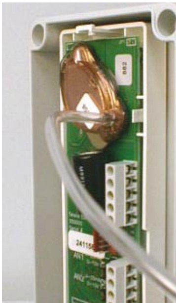
Figure 1: Test gas tube connected to the sample cell test gas input nipple.
