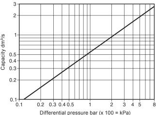
If the temperature of the air differs from 16°C, the discharge capacity from the graph can be corrected by miltiplying it by the following equation:
