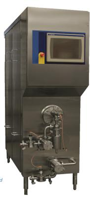
The shown freezer is with optional 3A approved seat valves. Standard is butterfly valves.
