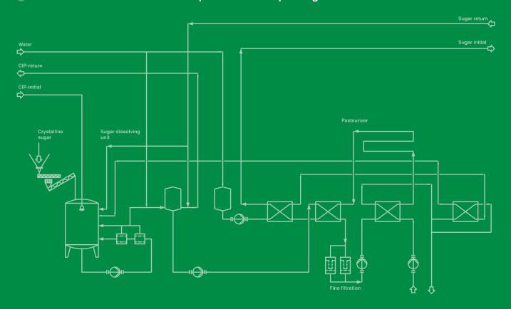
The INDAG sugar dissolving units facilitate the residue-free production of liquid sugar. The continuous dissolving of sugar saves time and is perfectly suited to high performance requirements. The integrated, fully-automated brix measurement ensures the constant brix value of the liquid sugar.
