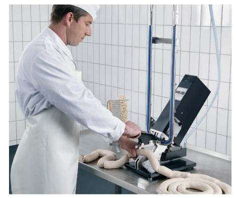
The DCD 600 securely closes all sheep, pork and beef rounds as well as synthetic casings up to calibre 60 mm
