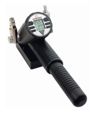
The pressure calibrator is used for precise monitoring and adjustment of pressure gauges and transmitters. It is equipped with a precision manometer. A fine adjusting screw and a valve complete this portable device.
