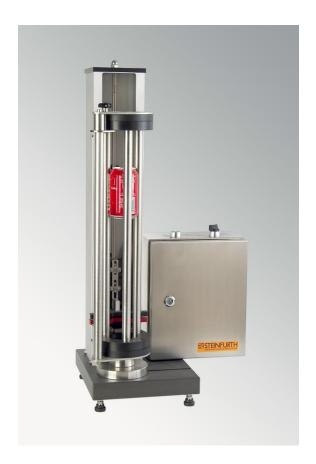
The Drop / CART Tester is a testing device designed to support two different beverage can stability tests: Drop Test and Can Abuse Resistance Test (CART). The Drop test includes repeated dropping of a specimen can onto a plain anvil plate from ever increasing heights. CART includes repeated dropping of a specimen can onto an anvil plate different from that used for the drop test, but from a fixed height.
