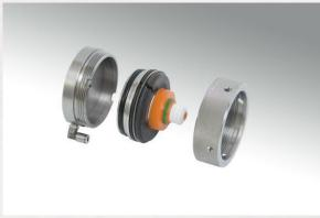
The PET bottle finish fixture is a means for pressure testing closures on finishes of existing PET bottles if a preform isn't available for that purpose. It is designed for use inside the safety tank of the Steinfurth Closure Tester V4. It is made entirely of stainless steel and other waterresistant materials.
