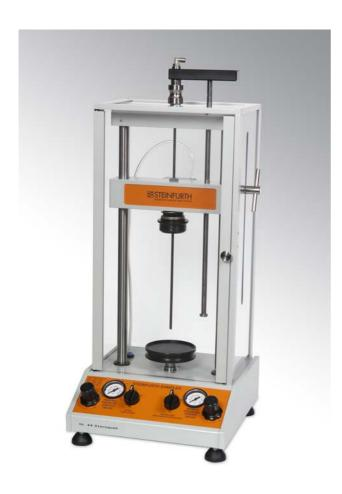
The Steinfurth Sampler pierces and pressurizes PET and glass bottles and cans. Piercing is performed pneumatically, so there is no need for great manual forces. The Steinfurth Sampler is suitable for gas analyses (e.g. oxygen, CO<sub>2</sub>...) and foam stability measurements.
