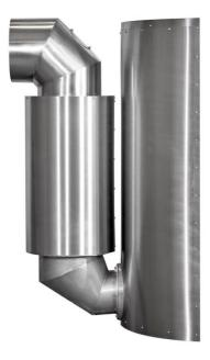
An economiser is a heat exchanger which utilizes the residual energy of the flue gases for heating of feed water. The economiser is the flue gas side connected between the steam boiler and the chimney. On the water side of the economizer between the boiler feed pump and the pressure element is connected. The water to be heated flows in counter-current to the flue gases to be cooled.
