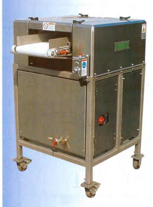
Bridge Machine Heavy Duty Con-Vey Cubers are designed to heavily tenderize or "macerate" large pieces of meat. The unit features large diameter blades that are independently air-spring loaded with adjustable stops to allow for different cutting options. The air-spring loaded blade action allows you to run different size pieces through the Cuber at the same time and maintain a consistent depth of cut.
