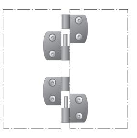
Right hinge. The right hinge half is fixed. The hatch or door opens from left to right.
