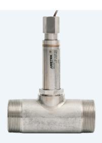
Model 851 Flushmount - with welded coupling in pipe for viscous media, slurries, or applications where parafin wax may build inside. Sensor can be easily removed to allow diaphragm steam cleaning as needed.
