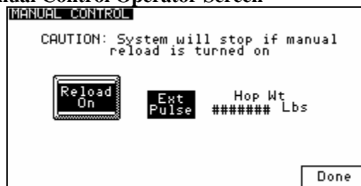
Figure 48: Typical Manual Control Operator Screen
