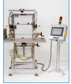
T4000 Dual Sensor Compression (DSC) System. Sensor has a cantilever design that suspends over the existing conveyor.
