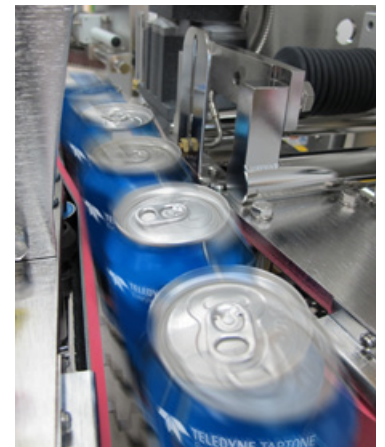
Cans being tested in TapTone T4000-FSB
