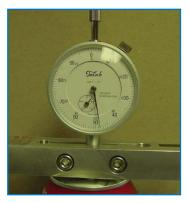
Good can with internal pressure of 23 psi from LN2 dosing. Deflection shows .052" from the chines to the rivet on the pull-tab.
