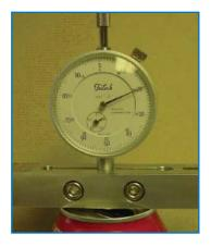
Flat can with no internal pressure. Deflection shows .080" from the chines to the rivet on the pull-tab. Center of can end has dropped from loss of internal pressure.
