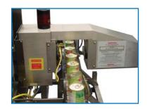
2. Down Can Sensor - used to detect cans that have fallen over on the line and were not inspected.
