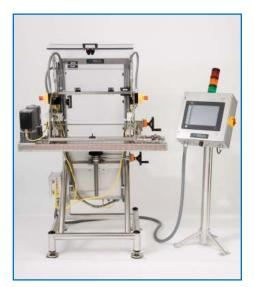
T4000 Dual Sensor Compression (DSC) System. Sensor has a cantilever design that suspends over the existing conveyor.
