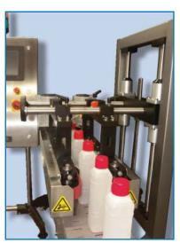
T-4000 Compression Controller and Sensor. Sensor has a cantilever design that suspends over the existing conveyor.
