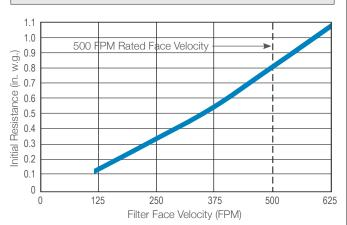
Filters are rated at 500 FPM filter face velocity. Recommended final resistance for all BioCel® M-Pak filters is 2" w.g.
