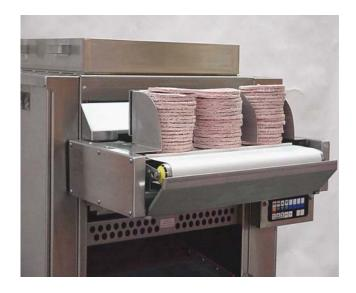
With **Autoloader**<sup>TM</sup> you can place 12 frozen hamburger patties in a stack and walk away! During peak time you can load up to 36 frozen patties and walk away!
