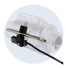
The VA Series valve can be provided with magnetically driven limit switches and an LED indicator. The limit switches are fixed to the outside of the unit. The magnets are situated inside the valve and must be installed during valve assembly, for this reason the switches must be requested at the time of order.
