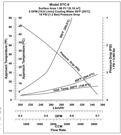
Performance data shows approach temperature (outer tube inlet + approach temp. = inner tube outlet temp.) for three inner tube inlet temperatures and various flow rates. Data based on thermal properties of water. Cooling water 95°F (35°C) @ 5 GPM (18.9 L/min). Pressure drop <18 psi (1.2 bar). Consult factory for other fluids flow rates and pressure drops.
