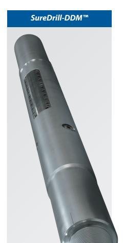
APS's Drilling Dynamics Monitor (DDM™)\* measures and records weight on bit, torque on bit, bending on bit, internal and annular pressure and temperature. Captured data may be transmitted in real time via APS's SureShot™ MWD/LWD system, or stored in the DDM's downhole memory for later download and analysis.
