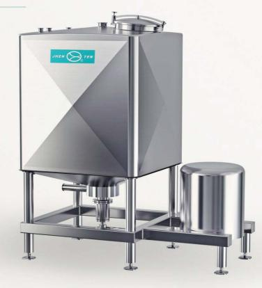
Square High Shear Emulsification Tank use square single layer stainless steel, and the inner wall of the tank body is made of circular transition, , no dead corner, easy to clean; and the bottom with mechanical emulsification.
